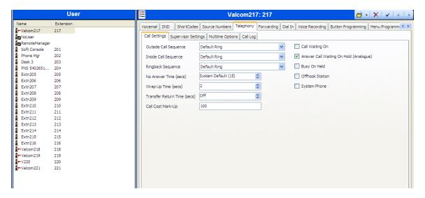
7. Click the Supervisor Settings sub-tab. If the "Force Authorisation" option was selected in Step 2, enter the Login Code for this User. The Login Code is the password that will be used by the Valcom device during the SIP registration process. When finished, click the OK button at the bottom of the window.
